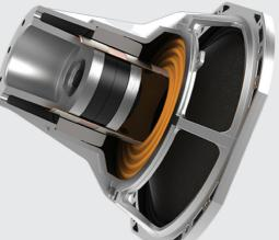
The SRX900's 2432H-3 compression driver features a neodymium magnet structure, 3-inch titanium diaphragm and a 1.5-inch exit, for crisp transients, superior dynamic range and extended sensitivity beyond 10 kHz, for truly linear high-frequency response at any output level.
